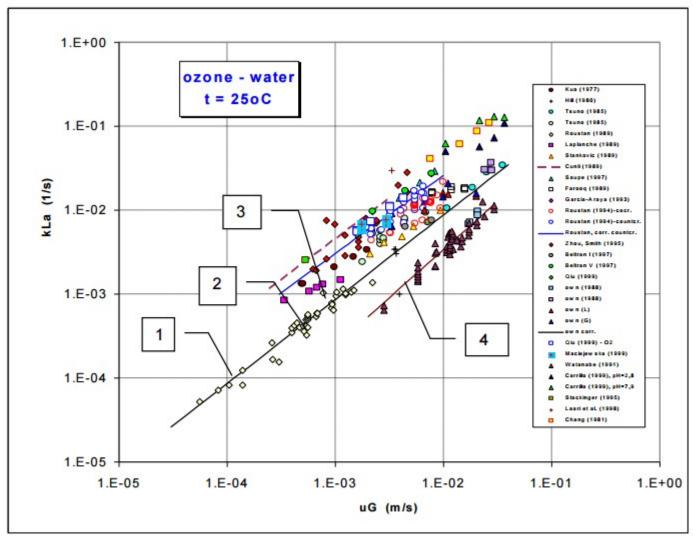
Experimental data of  $k_L a$  vs.  $u_G$  in the bubble columns:
